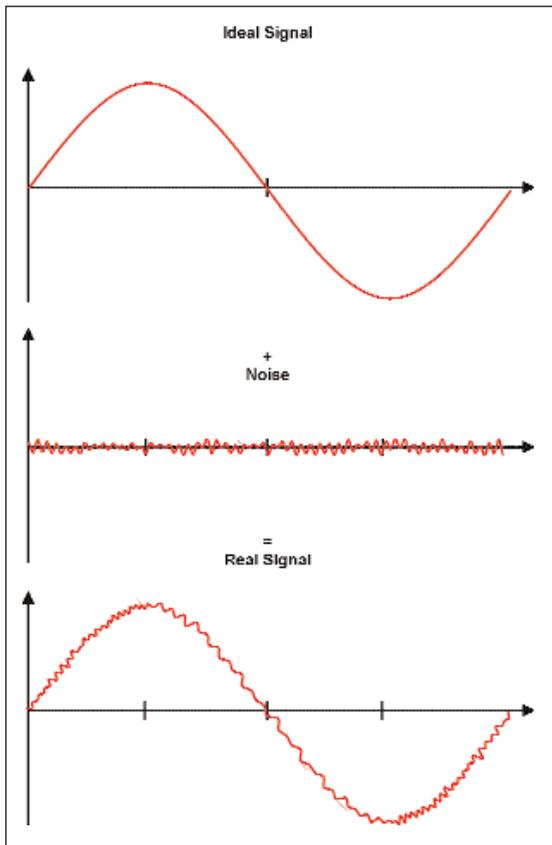
**Figure 13-6** Each device in the path adds noise to the final sound
