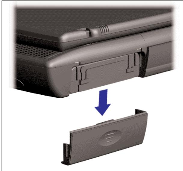
**Figure 16-6** Removing a drive from a modular bay
